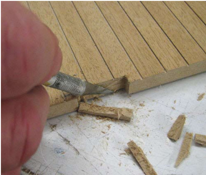
Cutting an Electrification Slot before building
