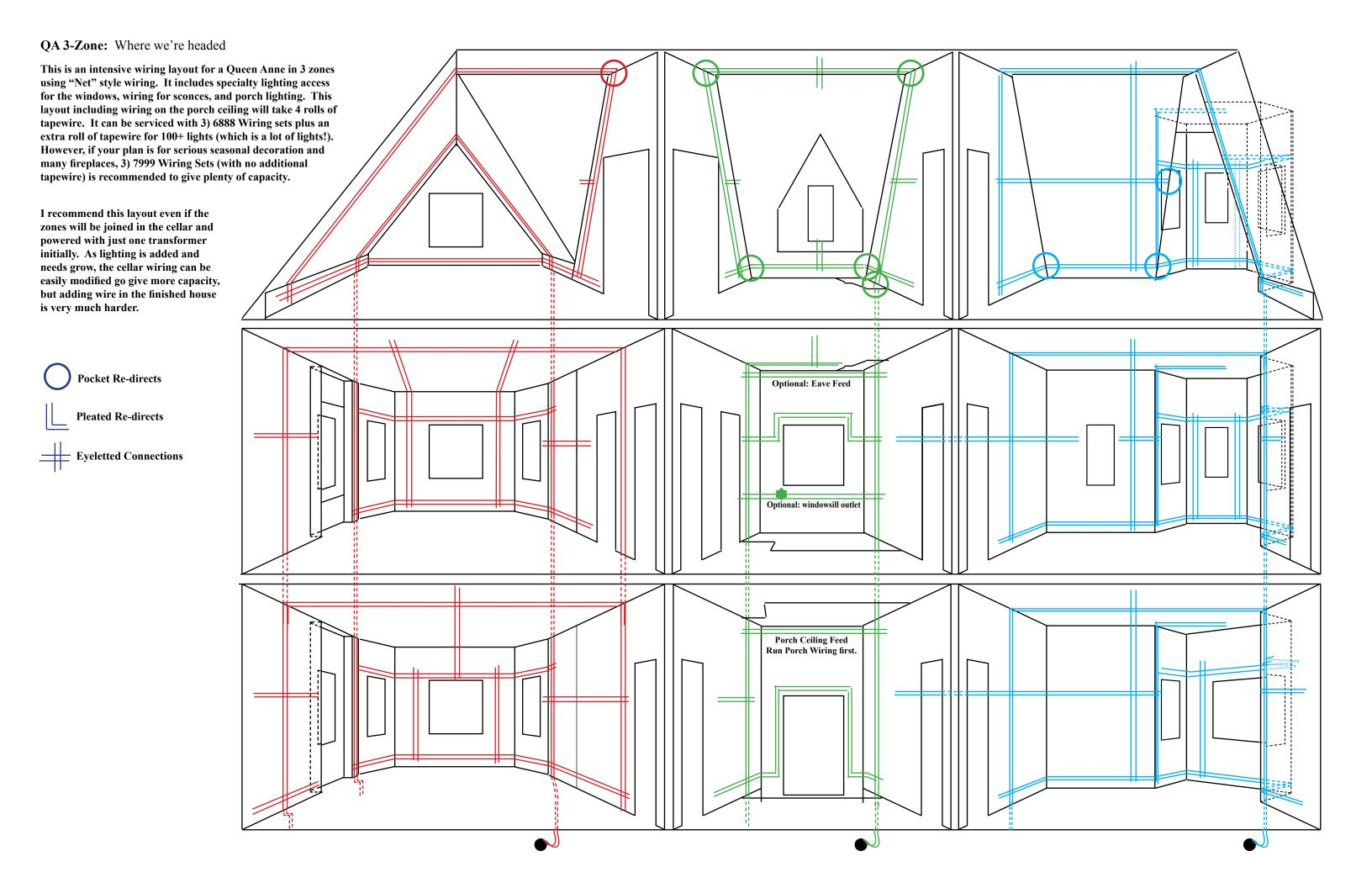
... As you build: The doubled circles on this page show electrification slots for running tapewire from floor-to-floor.
