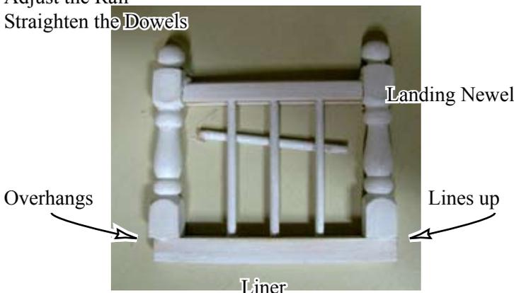
3: Glue Landing Newels to the Liner and Rail. The Newel is thicker than the Liner, and overhangs toward you. The right Newel in this photo lines up with the Liner; the left Newel overhangs the end.
