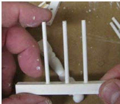
1: Glue Dowels into the 3<sup>7</sup>/<sub>16</sub> Liner's holes.
