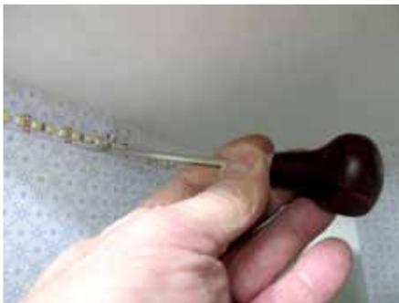
Drive the last-little-bit with an awl to avoid hitting the emitter
